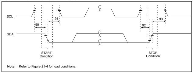
TABLE 21-15: I<sup>2</sup>C BUS START/STOP BITS REQUIREMENTS (SLAVE MODE)
