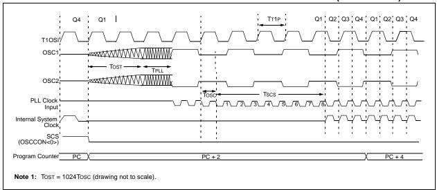
If the main oscillator is configured in the RC, RCIO, EC or ECIO modes, there is no oscillator start-up time-out. Operation will resume after eight cycles of the main oscillator have been counted. A timing diagram, indi-
