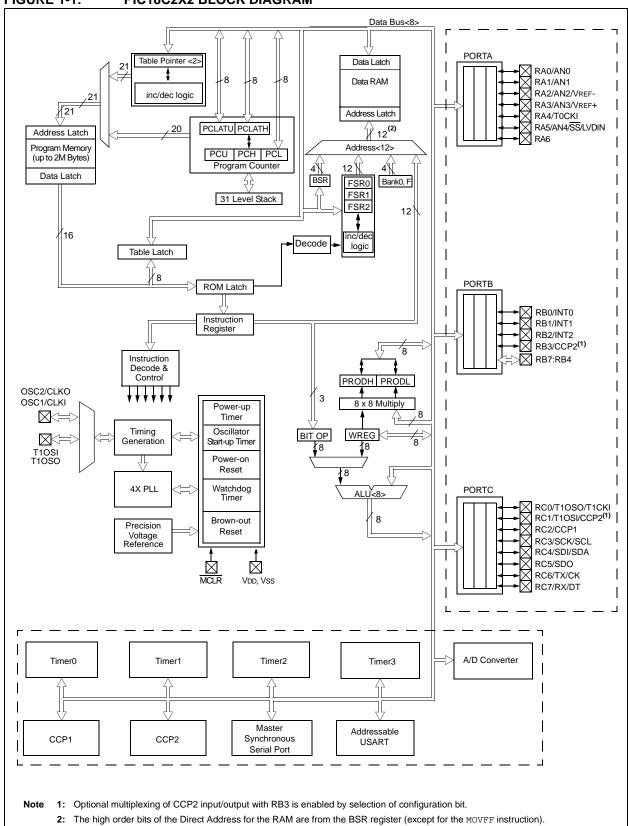
3: Many of the general purpose I/O pins are multiplexed with one or more peripheral module functions. The multiplexing combinations
