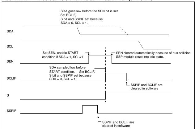
FIGURE 14-25: BUS COLLISION DURING START CONDITION (SCL = 0)
