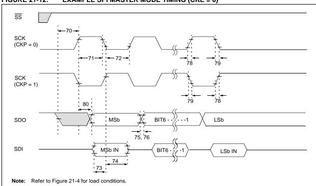
FIGURE 21-12: EXAMPLE SPI MASTER MODE TIMING (CKE = 0)
