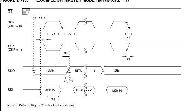
FIGURE 21-13: EXAMPLE SPI MASTER MODE TIMING (CKE = 1)
