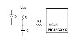
Note 1: External Power-on Reset circuit is required only if the VDD power-up slope is too slow.
