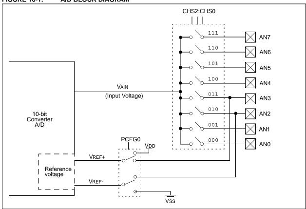
The value that is in the ADRESH/ADRESL registers is not modified for a Power-on Reset. The ADRESH/ADRESL registers will contain unknown data after a Power-on Reset.
