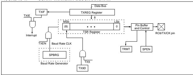
FIGURE 15-2: ASYNCHRONOUS TRANSMISSION
