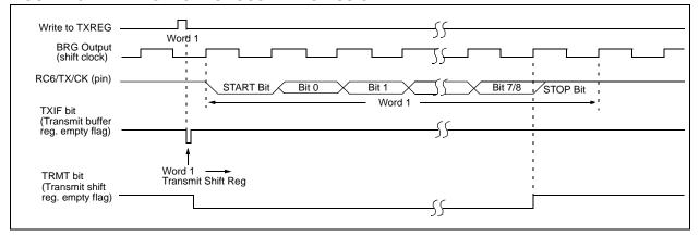
FIGURE 15-3: ASYNCHRONOUS TRANSMISSION (BACK TO BACK)
