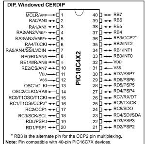
Note: Pin compatible with 40-pin PIC16C7X devices.
