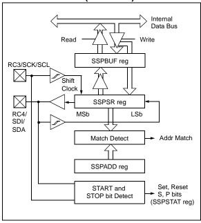
The MSSP module has six registers for  $I^2C$  operation. These are the:
