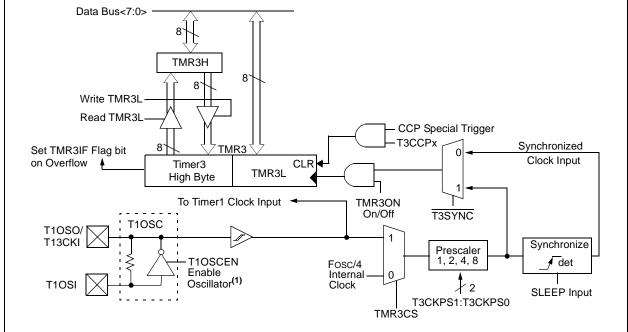
Note 1: When enable bit T1OSCEN is cleared, the inverter and feedback resistor are turned off. This eliminates power drain.
