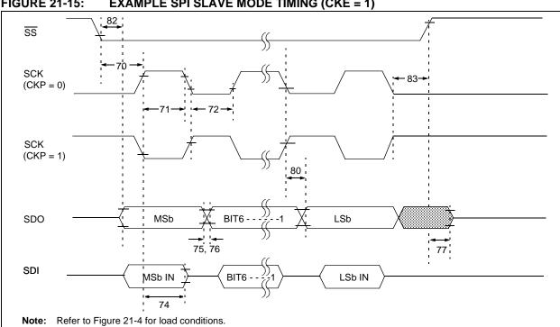
FIGURE 21-15: **EXAMPLE SPI SLAVE MODE TIMING (CKE = 1)**
