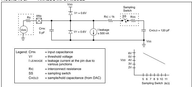
To calculate the minimum acquisition time, Equation 16-1 may be used. This equation assumes that 1/2 LSb error is used (1024 steps for the A/D). The 1/2 LSb error is the maximum error allowed for the A/D to meet its specified resolution.
