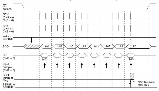
FIGURE 14-6: SPI MODE WAVEFORM (SLAVE MODE WITH CKE = 1)
