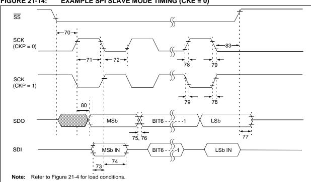
FIGURE 21-14: **EXAMPLE SPI SLAVE MODE TIMING (CKE = 0)**
