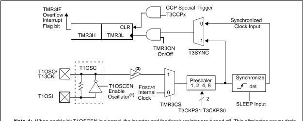
Note 1: When enable bit T10SCEN is cleared, the inverter and feedback resistor are turned off. This eliminates power drain.
