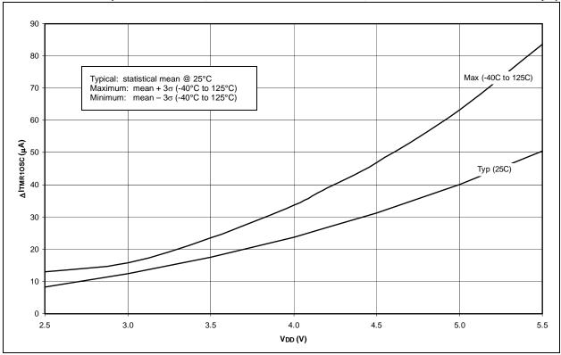
FIGURE 22-16: TYPICAL AND MAXIMUM AIWDT vs. VDD OVER TEMPERATURE (WDT ENABLED)
