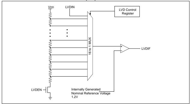
The LVD module has an additional feature that allows the user to supply the trip voltage to the module from an external source. This mode is enabled when bits LVDL3:LVDL0 are set to 1111. In this state, the comparator input is multiplexed from the external input pin LVDIN (Figure 17-3).
