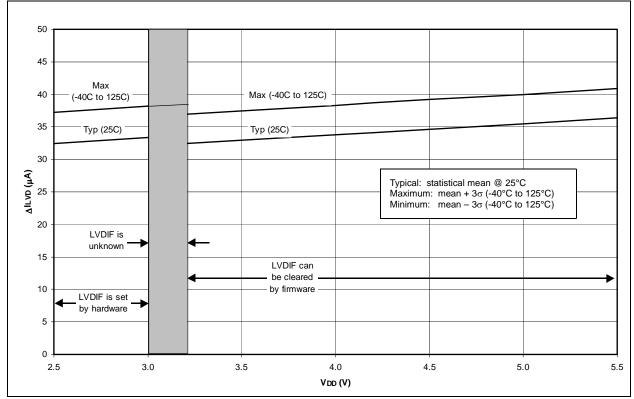
FIGURE 22-19: Allvd vs. Vdd OVER TEMPERATURE (LVD ENABLED, VLvd = 4.5V - 4.78V)
