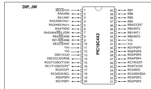
Note: Pin compatible with 40-pin PIC16C7X devices.
