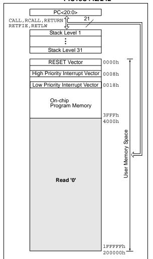
FIGURE 4-2: PROGRAM MEMORY MAP AND STACK FOR PIC18C452/252
