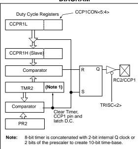
A PWM output (Figure 13-4) has a time-base (period) and a time that the output stays high (duty cycle). The frequency of the PWM is the inverse of the period (1/period).
