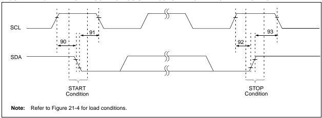
TABLE 21-17: MASTER SSP I<sup>2</sup>C BUS START/STOP BITS REQUIREMENTS
