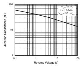
Fig. 5 - Typical Junction Capacitance
