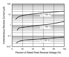
Fig. 4 - Typical Reverse Characteristics
