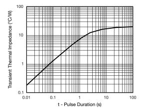
Fig. 6 - Typical Transient Thermal Impedance
