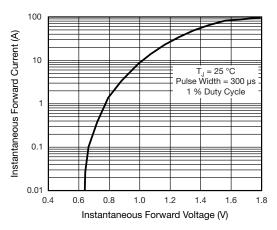
Fig. 3 - Typical Instantaneous Forward Characteristics
