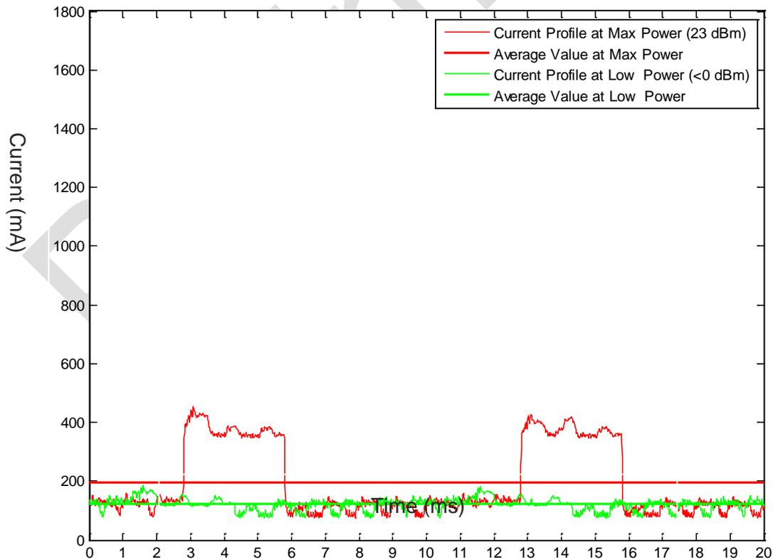
Current Consumption in GPRS 1 slot TX
