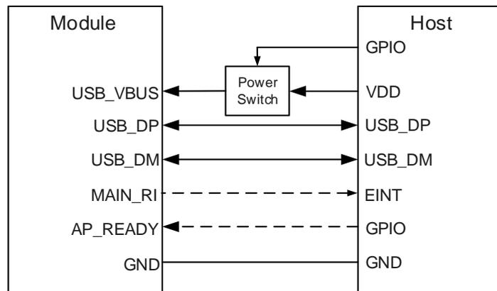
**Figure 6: Sleep Mode Application without Suspend Function**
