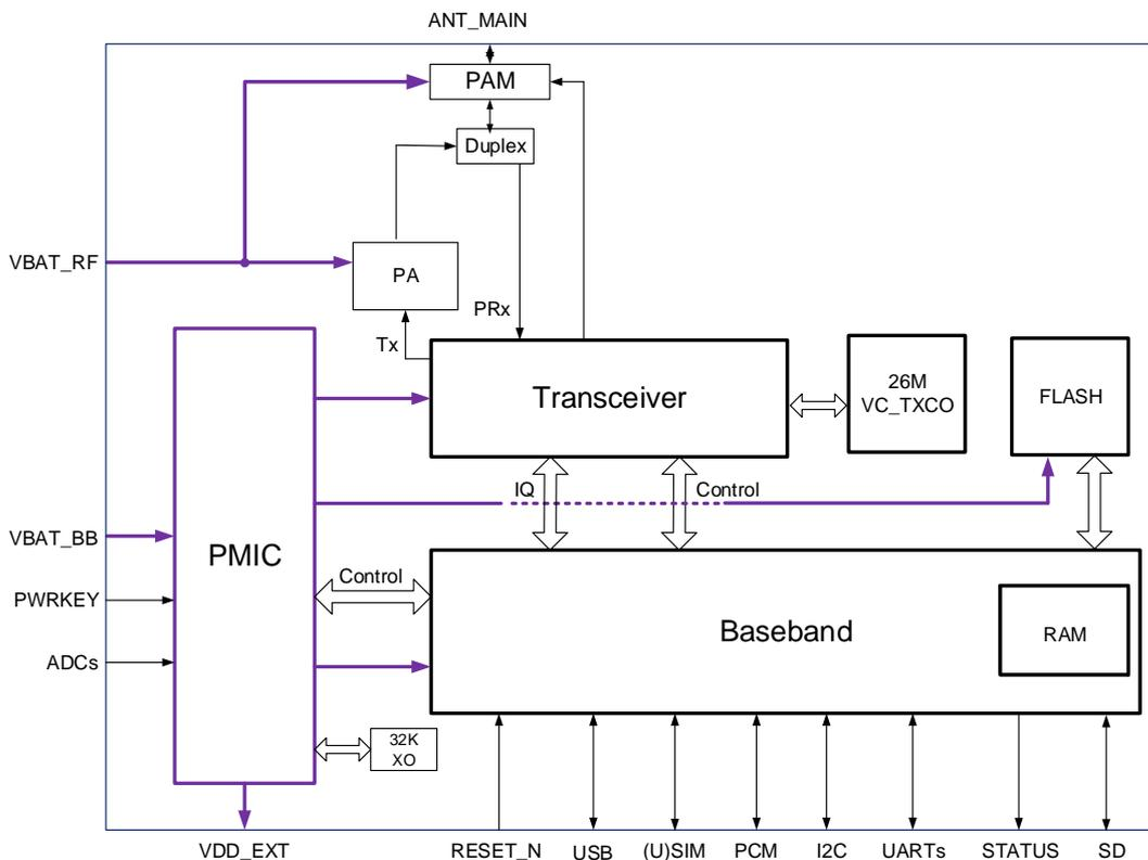
**Figure 1: Functional Diagram**
