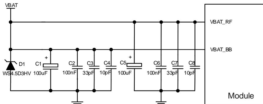
**Figure 8: Star Structure of the Power Supply**
