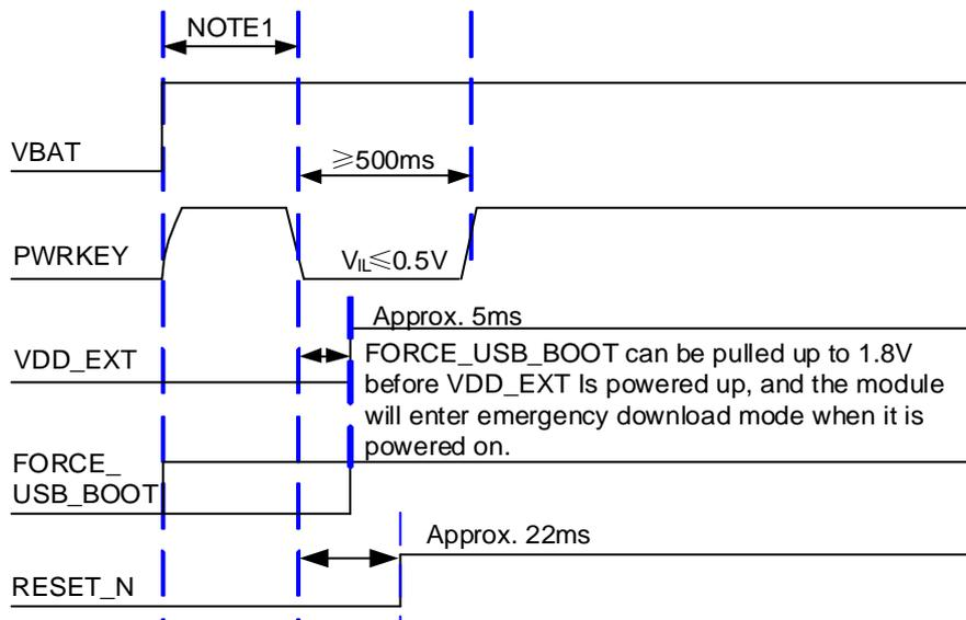
Figure 28: Timing Sequence for Entering Emergency Download Mode
