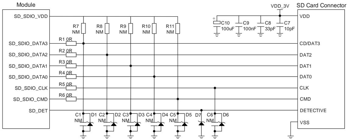
**Figure 24: Reference Circuit of SD Card Interface**
