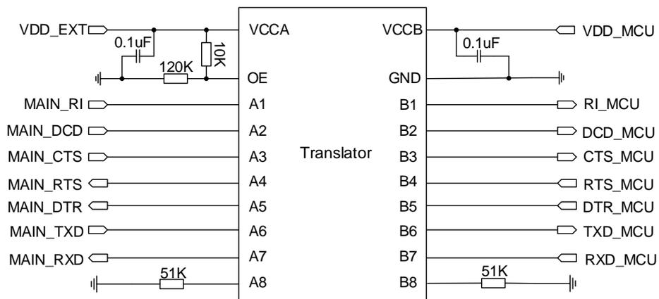
**Figure 20: Reference Circuit with a Level Translator Chip**
