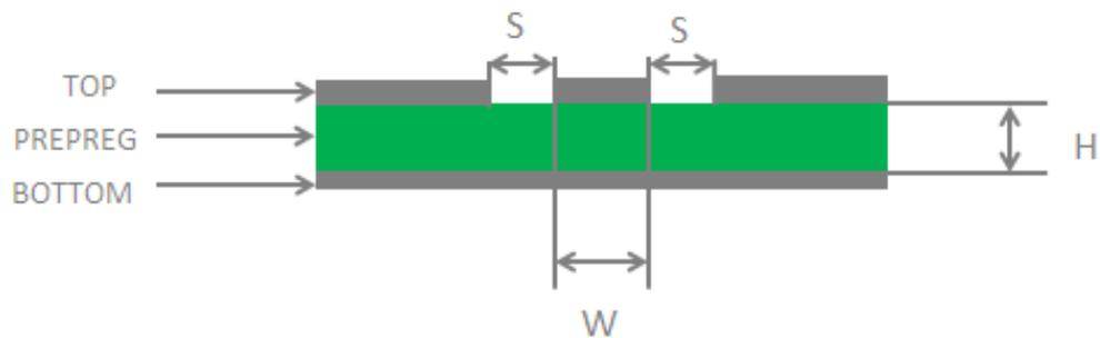
Figure 31: Coplanar Waveguide Design on a 2-layer PCB
