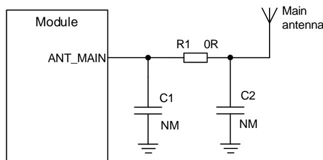
**Figure 29: Reference Circuit of RF Antenna Interface**
