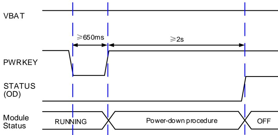
Figure 13: Timing of Turning off the Module
