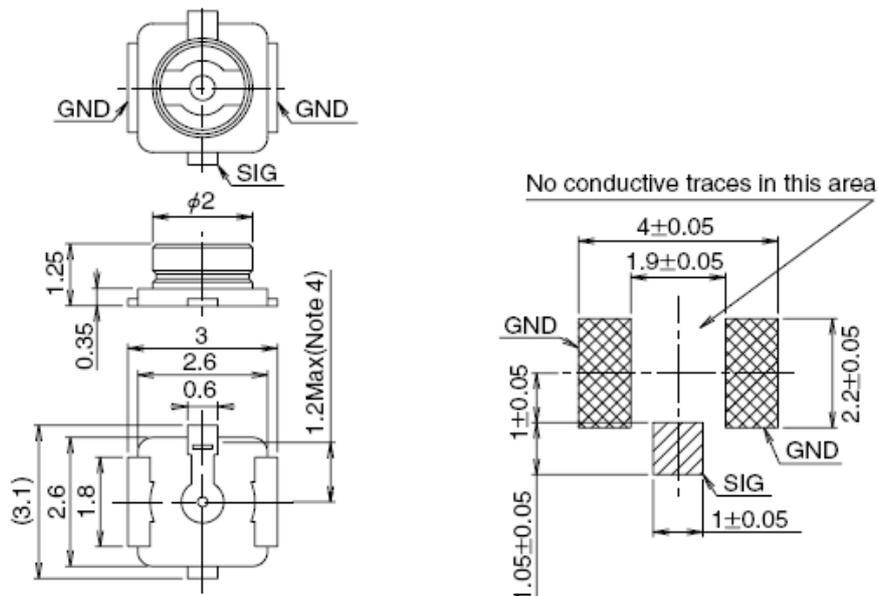
**Figure 34: Dimensions of the U.FL-R-SMT Connector (Unit: mm)**
