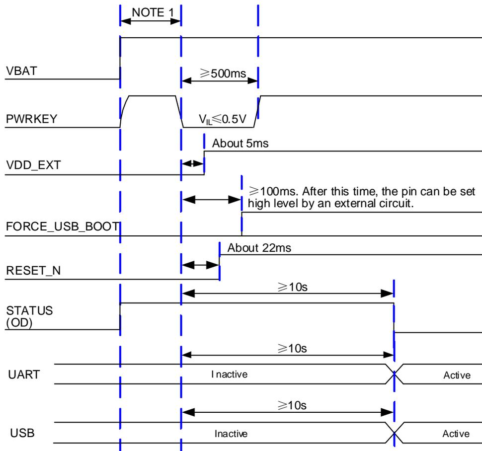
**Figure 12: Timing of Turning on the Module**
