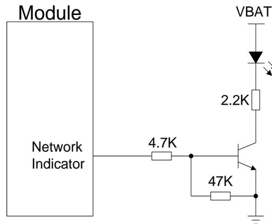
**Figure 25: Reference Circuit of the Network Status Indication**
