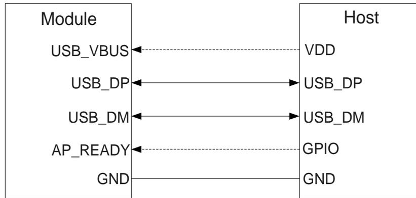
**Figure 4: Sleep Mode Application with USB Remote Wakeup**
