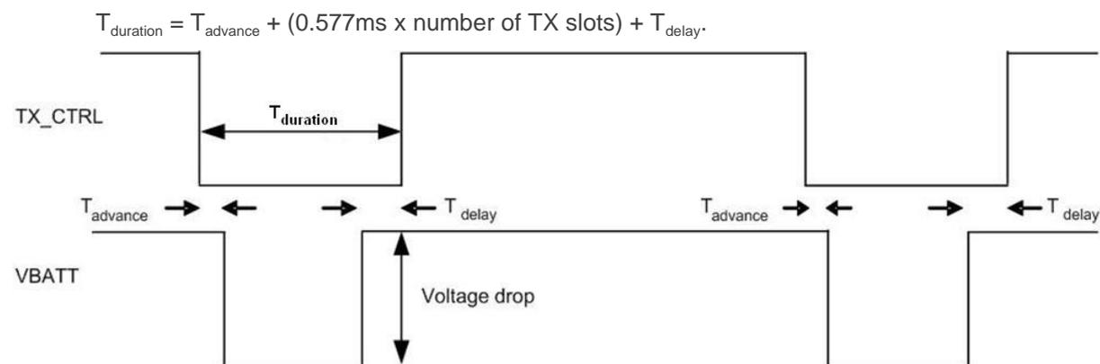
Figure 36. TX\_CTRL State During TX Burst
