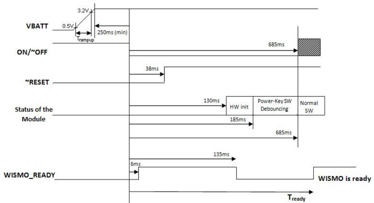
Figure 31. Power-ON Sequence (no PIN code activated)
