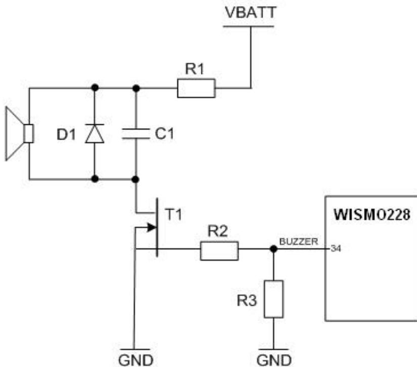
Figure 28. Example of a BUZZER Implementation
