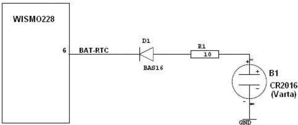
Figure 34. RTC Supplied by a Non Rechargeable Battery
