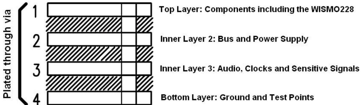
Figure 44. PCB Structure Example for the Application Board
