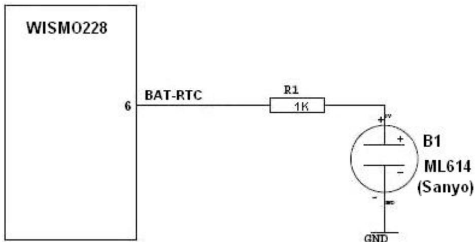
Figure 35. RTC Supplied by a Rechargeable Battery Cell
