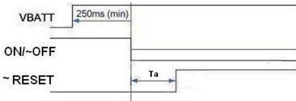
Figure 38. Reset Timing
