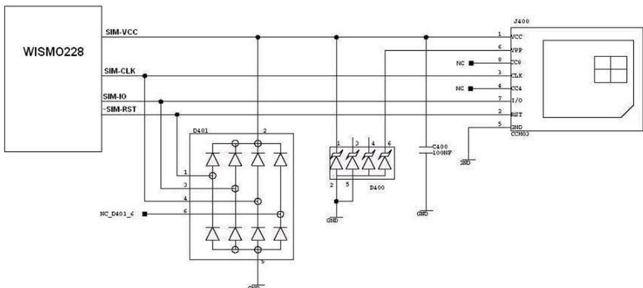
Figure 12. Example of a SIM Socket Implementation
