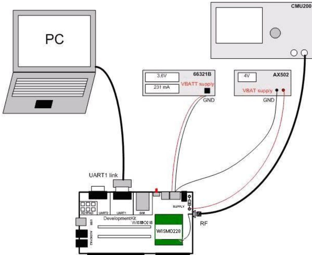
Figure 42. Typical Hardware Configuration
