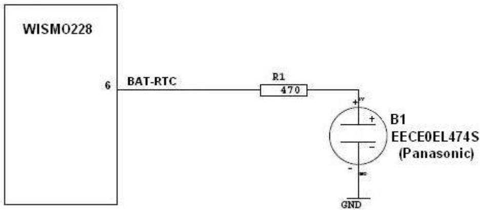
Figure 33. RTC Supplied by a Gold Capacitor
