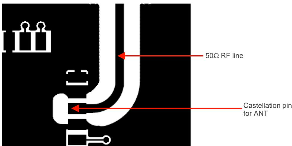
Figure 41. Example of a  $50\Omega$  RF Line
