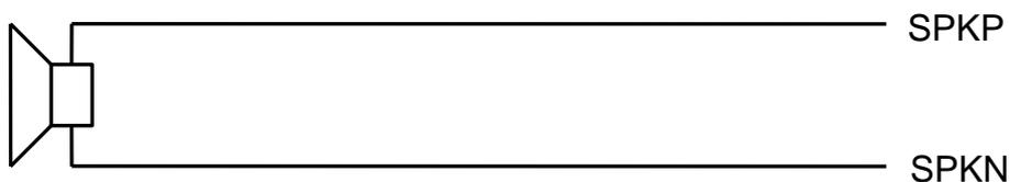
Figure 19. Example of a Differential Speaker Connection
