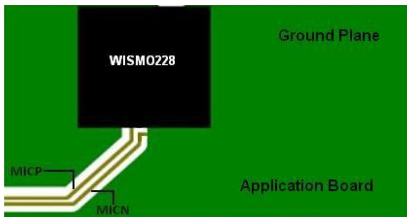
Figure 24. Single-Ended Audio Connection
