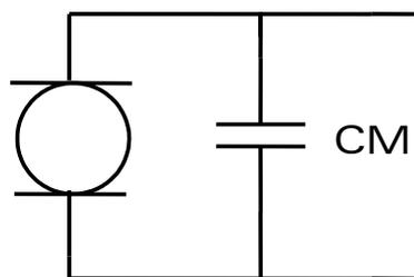
Figure 21. Capacitor Soldered in Parallel to the Microphone
