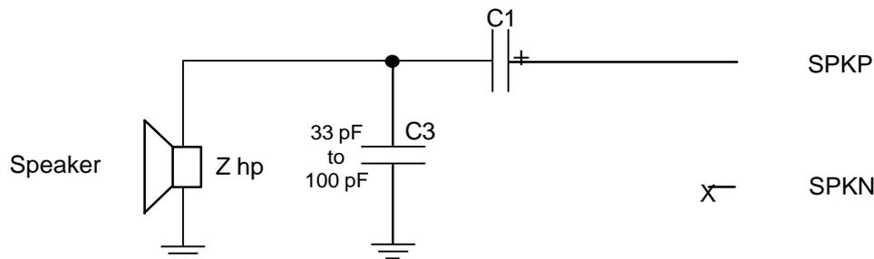
Figure 20. Example of a Single-Ended Speaker Connection
