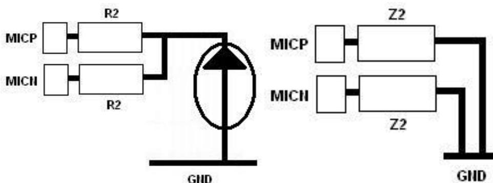
Figure 13. DC and AC Equivalent Circuits of MIC
