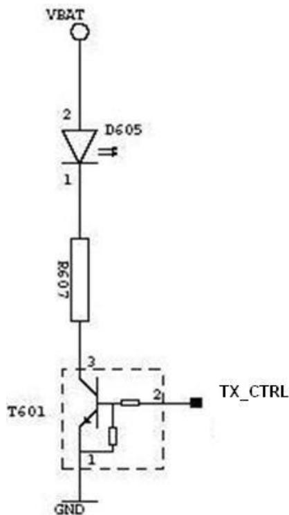
Figure 37. Example of a TX Status Implementation
