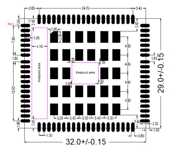
Figure 39: Recommended Footprint (Top View)
