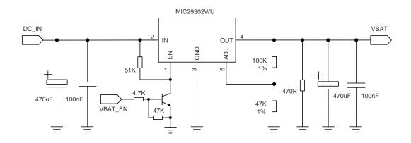
Figure 9: Reference Circuit of Power Supply
