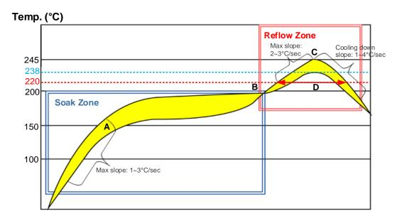
Figure 42: Reflow Soldering Thermal Profile
