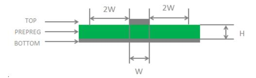
Figure 30: Microstrip Design on a 2-layer PCB
