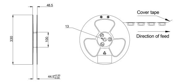
Figure 43: Tape and Reel Specifications
