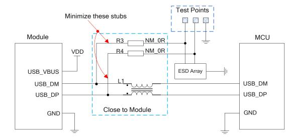
Figure 19: Reference Circuit of USB Application
