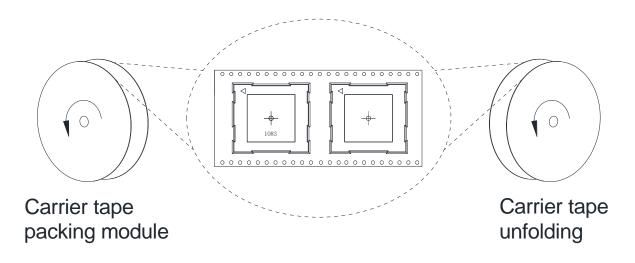
Figure 44: Tape and Reel Directions
