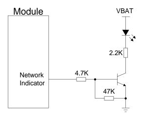
Figure 25: Reference Circuit of the Network Status Indication
