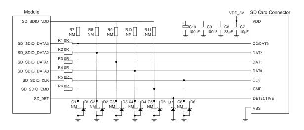
The following figure shows a reference design of the SD card interface.
