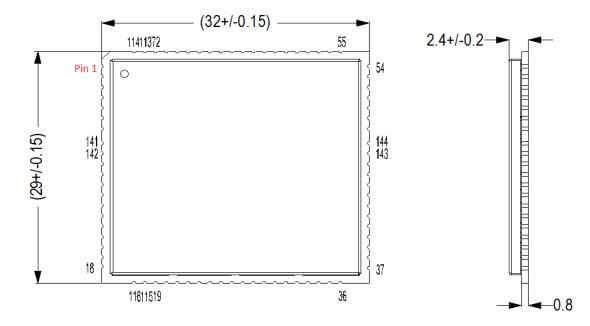
Figure 37: Module Top and Side Dimensions
