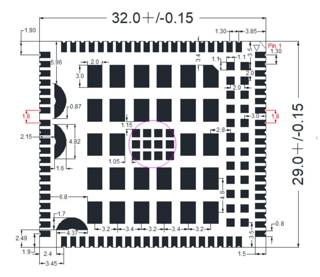
Figure 38: Module Bottom Dimensions (Bottom View)
