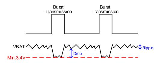
Figure 7: Power Supply Limits during Burst Transmission
