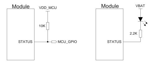
Figure 26: Reference Circuits of STATUS
