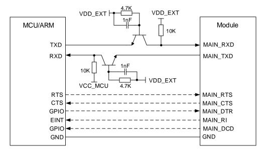
Figure 21: Reference Circuit with a Transistor Circuit
