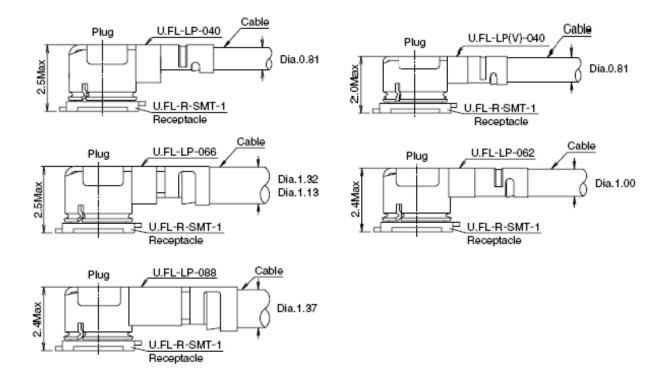
Figure 36: Space Factor of Mated Connectors (Unit: mm)
