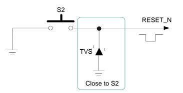
Figure 15: Reference Circuit of Resetting the Module by Using Button
