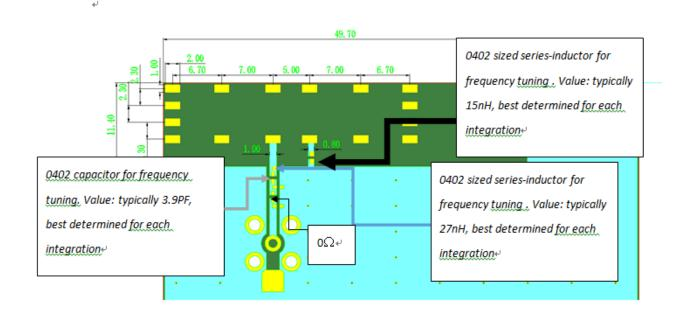
The antenna requires a matching circuit that must be optimized for each product. The matching circuit will require up to six components and the following circuit should be designed into the host PCB. Not all components may be required but should be included as a precaution. The matching network must be placed close to the antenna feed to ensure it is more effective in tuning the antenna.
